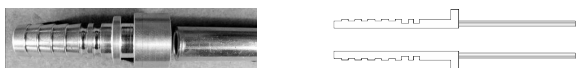
Figure 1. a) The components for friction welding, nipple and pipe, b) Joint configuration
