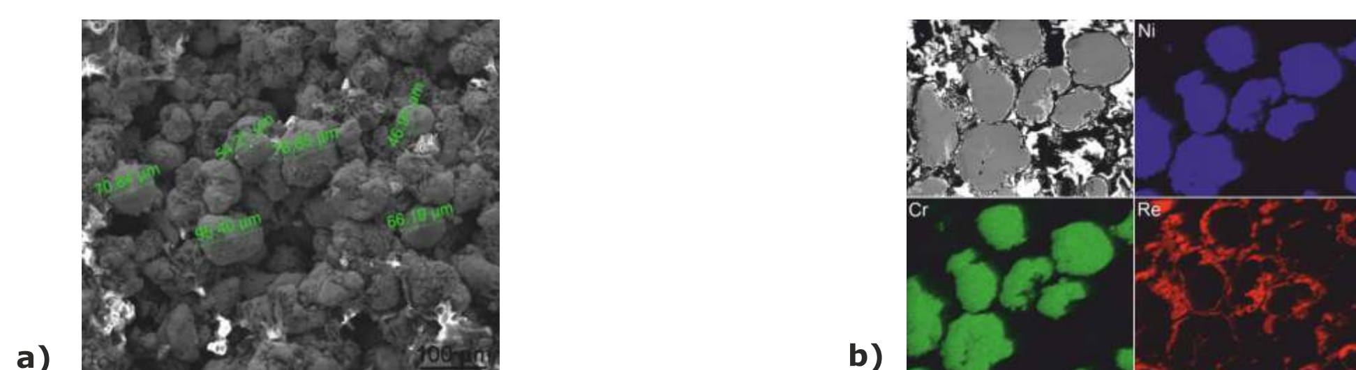
Figure 1. Ni20%Cr + 20%Re powder for plasma spraying, a) general view, b) EDS analysis – Ni (blue), Cr (green), Re (red)
