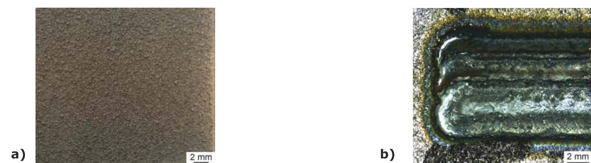
Figure 2. General view of sprayed surface, a) after spraying, b) after laser remelting
